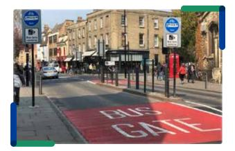
A Bus Gate is a sign-posted short length of stand-alone bus lane. This short length of road is restricted exclusively to buses, taxis and cyclists plus emergency vehicles. It facilitates bus priority by removing general through traffic along the overall road where the bus gate is located. General traffic will be directed by signage to divert away to other roads before they arrive at the bus gate. To see an animation of a how a Bus Gate will work, please visit our website www.busconnects.ie.
